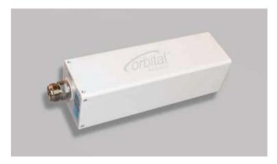
This Ka-band low noise block downconverter (LNB) uses multiple local oscillators to let you switch between different Ka frequency bands in the 19.20 to 21.20 GHz range. It provides user bandwidth of up to 1 GHz and offers exceptional performance for commercial and military satellite communication (SATCOM) applications.
