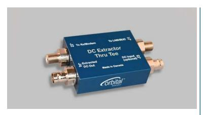
The Orbital DC Power Extractor Thru Tee (DET-25/40) taps off the incoming DC from the modem and splits it between the combined port to the LNB/BUC and a separate DC-only port – so you can power an external device at the antenna. It also acts as a bias tee thruplexer (thru tee) and filters L-band, 10 MHz and DC signals.
