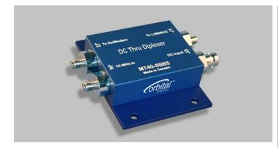
The Orbital DC Thru Diplexer (DTD-10) is a bias tee thruplexer that inserts a high-quality 10 MHz source into your LNB or BUC – in addition to passing both L-band and DC power from the modem with very low insertion loss. This small and compact device is easy to mount, can be used outdoors, and can be customized with any connector.
